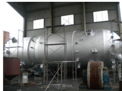
变换炉 Transform Furnace
