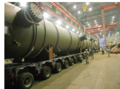
低温甲醇洗涤塔 Low Temperature Methanol Wash Tower
